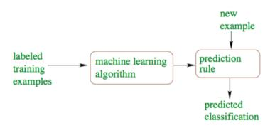
Learning a function that maps an input to an output based on example input-output pairs
